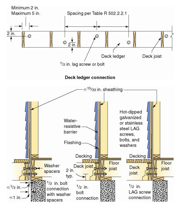
703.8 Requires corrosion-resistive flashing be provided in the exterior wall envelope in such a manner as to prevent entry of water into the wall cavity or penetration of water to the building structural components where porches, decks or stairs are attached to a wall or floor assembly of wood-frame construction.
